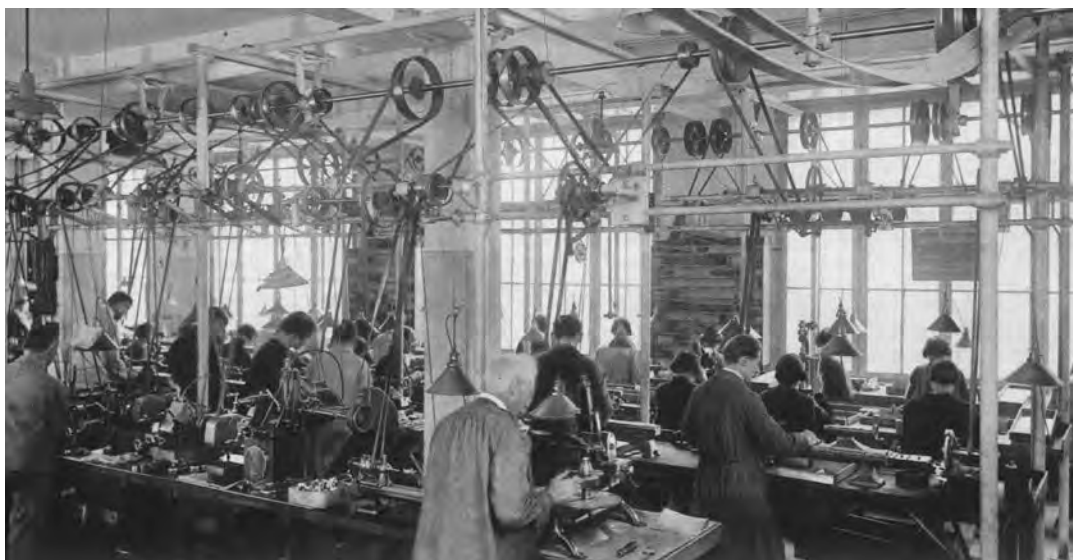
Production hall around 1935 with transmission belts to the workstations
