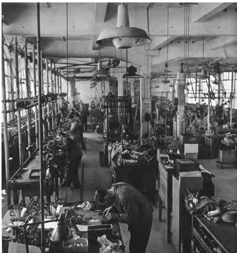
Production hall around 1935 with transmission belts to the workstations
